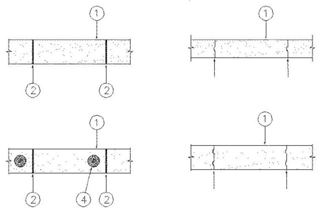
1. **Precast Autoclaved Aerated Concrete Blocks** — Min 4 in. thick by min 7-7/8 in. high by min 23-5/8 in. long blocks for use in 4 hr nonbearing wall assemblies. Min 6 in. thick by min 7-7/8 in. high by min 23-5/8 in. long blocks for use in 4 hr bearing wall assemblies. Min 3 in. thick by min 7-7/8 in. high by min 23-5/8 in. long blocks for use in 2 hr nonbearing wall assemblies. See Item 4 for minimum block thickness when cores are present.
