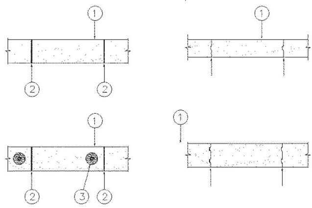
1. **Precast Autoclaved Aerated Concrete Blocks** — Nom 8 in. thick by 24 in. high by 40 in. long blocks. **AERCON FLORIDA L L C** — AC-2, AC-4, AC-6
